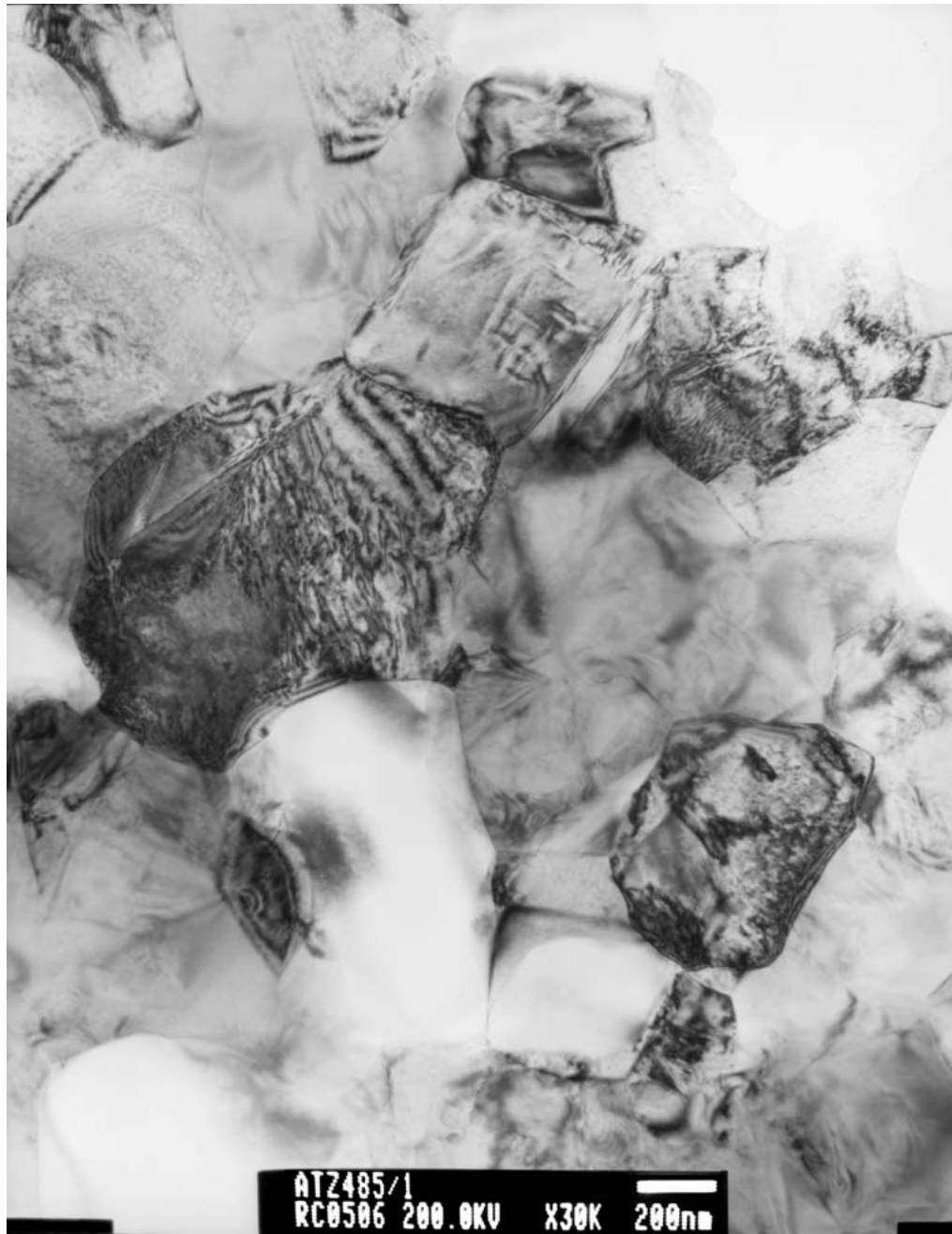
Figure 8 TEM image of the glass-free ATZ deformed at 1400°C with 52% deformation. High dislocation density and low-angle grain boundaries are visible within the Y-TZP grains.
